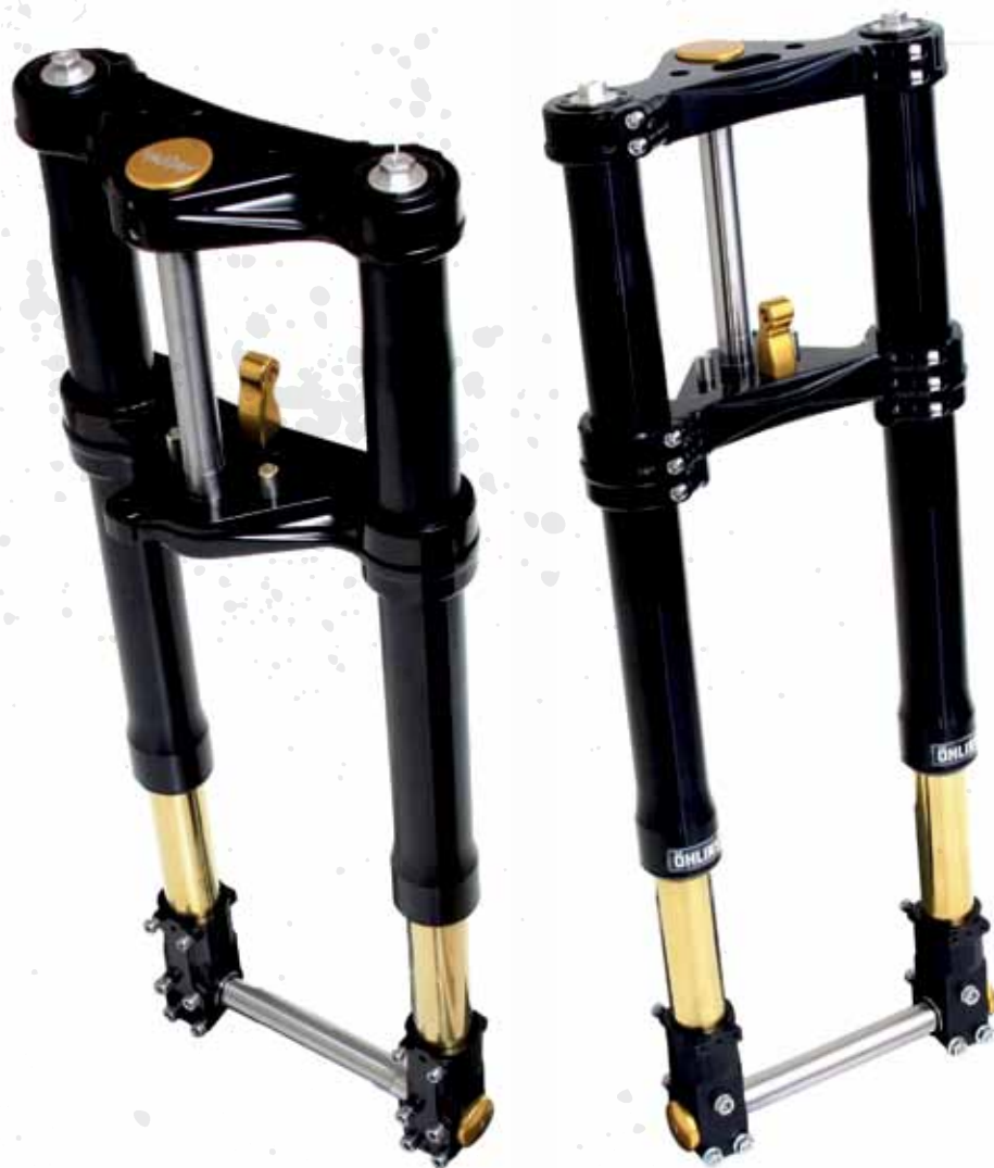
Indianapolis triple trees black anodized with OHLINS front forks.
