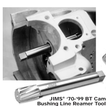
Use to line ream cam cover bushing to size from inner cam bearing on an unassembled '70-'99 single-cam engine. Finish size will be about .0008"-.0015" over the cam journal. #758-845
