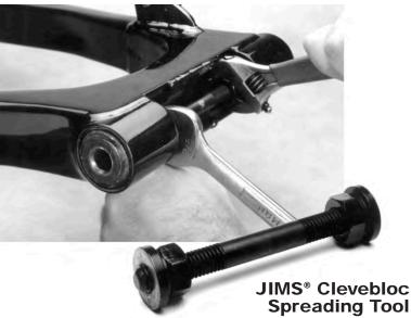
Use to install the swing arm in all FXR and '80-'01 FLT/HT models. This tool will spread the swing arm cleveblocs allowing for installation of the swing arm. #758-707
