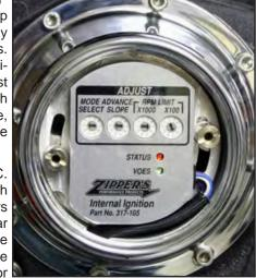
high compression engines. Engines equipped with nitrous or a turbo can configure the VOES input port to be used as a retard switch input instead, with up to 10° timing retard.
