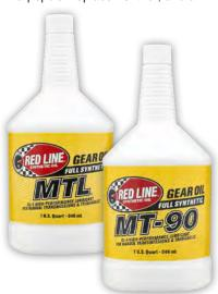
spec MS-9224. Red Line® MTL 70W80 GL-4 Gear Oil is safe for brass synchros, as it lacks the reactive sulfurs found in most GL-5 oils that cause damage. MTL 70W80 offers quicker shifts, eliminates notchy shifting (even when cold), and high performance gear protection. Satisifies the gear oil viscosity requirements of 70W, 75W, 80W, and motor oil viscosities of SAE 30, 10W30, and 5W30. Recommended for GL-1, GL-3, and GL-4 applications as well as where most special synchromesh fluids are specified.
