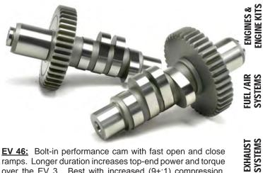
EV 46: Bolt-in performance cam with fast open and close ramps. Longer duration increases top-end power and torque over the EV 3. Best with increased (9+:1) compression. Power range 2600 to 6000+ RPM.
