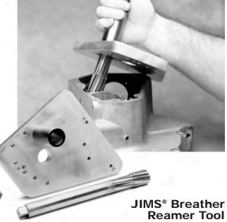
Repair a damaged breather hole without need to disassemble the cases. Using JIMS® Reamer Tool will ream a damaged breather hole to use a .030" oversize breather gear in less than an hours time. For '36-'99 single-cam BT. #758-706
