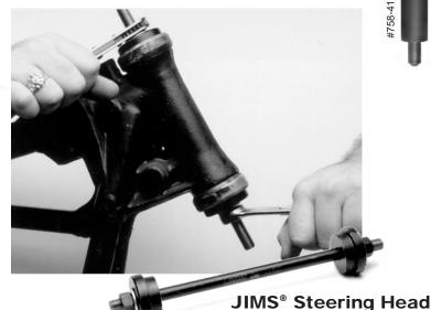
Use to install tapered steering head races and ball bearing cups into the frame on all models, straight and true. #758-725
