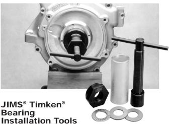
Use to install Timken bearings onto flywheel shafts and install flywheel assembly into left crankcase. Works best when used with JIMS® #758-660 1-7/8" socket (sold separately).
