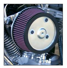
To make maximum power, you must Feed the Beast! Zipper's MaxFlow Flow Air Filter kits are designed to maximize available airflow and minimize intake turbulence at the entry point. We start with a fully machined, radius inlet billet backplate, and add special mounting and crankcase venting hardware that allows the installer to route breather venting externally (purchase vent filter separately). We top it off with our exclusive 2-3/4" deep-breathing MaxFlow filter element.
