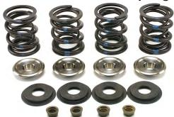
This valve spring kit is designed for use in Shovel or Pan engines with cam lifts of .500"-.580". It is a double spring kit with high strength titanium top collars, specially machined steel lowers and quality keys. Late Shovel heads ('79-up) that use .625" guide bores require a small-top guide such as our #588-500 series for proper lower collar fitment.
