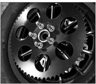
**Street O-Ring Kits** - Front sprockets are steel, rear are made from your choice of lightweight, extremely tough 7075-T6 aircraft quality aluminum, or steel in silver zinc or chrome finish.
