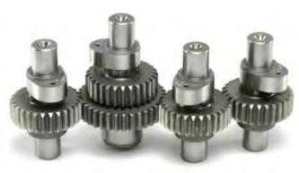
785V2: Offset tappet design - the original design of the venerable XL Pro-Stock-Top Gas Cams. This same profile has been used in many championship forms of racing. Net tappet lift is .485"; .785"@ valve with 1.62 rocker ratio. Increase rocker ratio for more valve lift.
