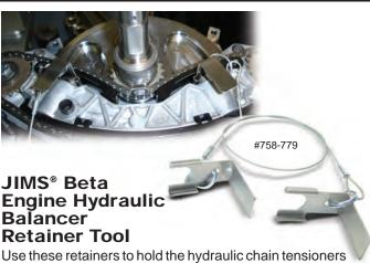
Use these retainers to hold the hydraulic chain tensioners in place when repairing all Beta engines. These are a "must have" tool for proper assembly or disassembly of the 'B' engine balancer system. #758-779
