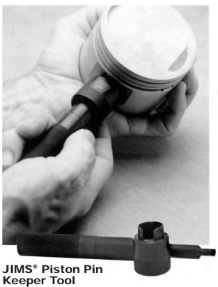
Use to install retaining ring in piston. This tool will install round circlip rings in one easy step without distorting ring, for the safest wrist pin retention possible. Use on all Big Twin 1983-present single cam and all Sportster® Late 1985-present. #758-623
