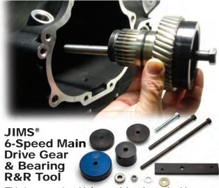
This is a complete kit for servicing the main drive gear and main bearing on the H-D® 6-speed transmission. This precision tool removes and installs both parts correctly without damaging the case. For 2006 FXD and all 2007-up Twin Cam® models. #758-900
