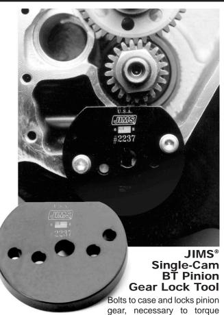
the pinion nut. Use on Big Twin '54-'99 single-cam engines. #758-237
