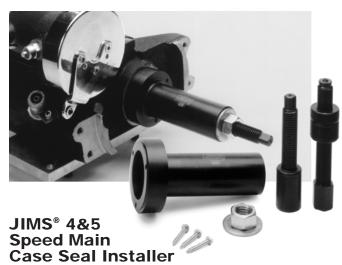
This tool will push the main drive case seal in as flat and straight as possible to .050" below housing for a no leak fit. Tool #758-642 includes the main tool components required and the seal installer for '41-'79 4-speeds. Order drivers for other year 4&5 speed transmissions separately.
